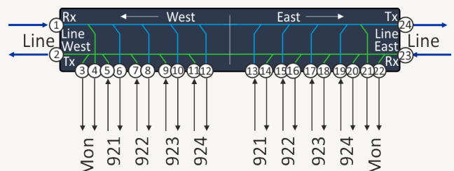
The port allocation and overlay example is for H-OADM2X4-921-924-4C. Note row dependent location of Tx and Rx ports. This is to match duplex connectors.
