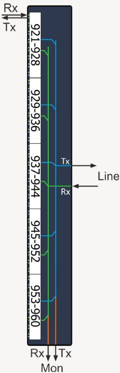
Client and Line signals entering the filter is denoted "Rx". Client and Line signals exiting the filter is denoted "Tx".
